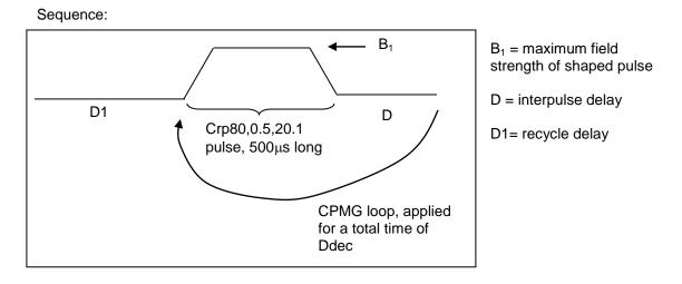
In standard cpmg sequences the 'decoupling time' Ddec is the length of the CPMG element (d20) and the inter-pulse delay is defined by 2\*D21.
