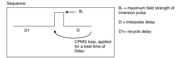
In standard cpmg sequences the decoupling time is the length of the CPMG element (d20) and the inter-pulse delay is defined as  $2^*D21$
