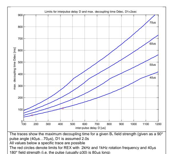
For a cpmg REX sequence with 2kHz and  $40\mu$ s pulse strength, a maximum decoupling time of about 50ms is allowed. (which means 2\* 25ms periods in the usual sequences).
