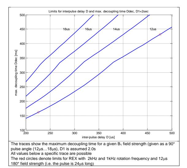
So, for a typical cpmg REX sequence with 2kHz and  $12\mu s$  pulse strength, a maximum decoupling time of about 150ms is allowed. (which means  $2^*$  75ms periods in the usual sequences)
