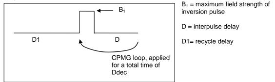
In standard cpmg sequences the decoupling time is the length of the CPMG element (d20) and the inter-pulse delay is defined by  $2^*D21$
