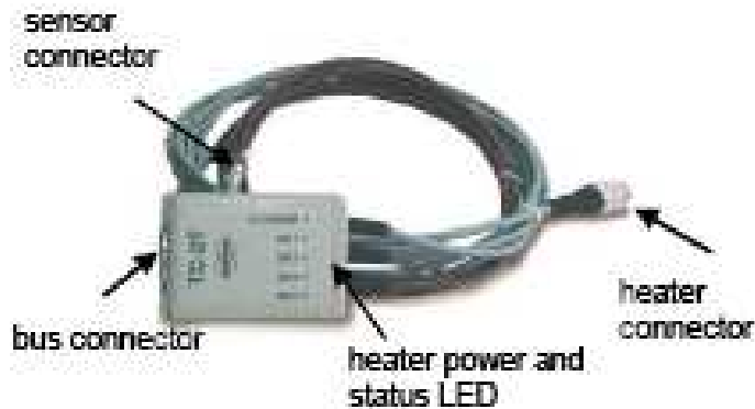
VTA for RT probes (thermocouple type T)
